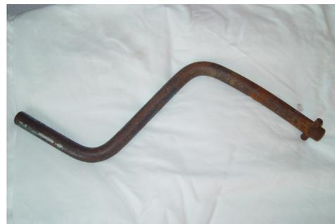
In the last newsletter, I mentioned that Randy Fehr was looking for an original-style crank (he found one at Hershey!) Eric Bloch came to the rescue on this one with a photo of the crank that came with his car years ago. Here are the specs: 14" long, 3/4" thick, chamfered ends, and the pin is 3/8" dia and 1 11/16 " long.
